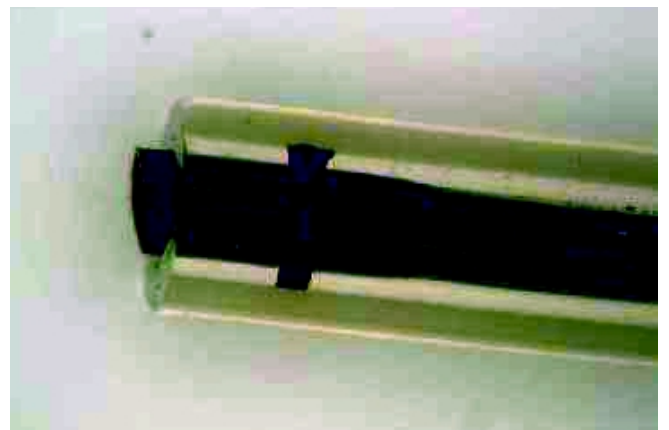
Figure 3: 0.012" wide circumferential weld on 0.005" wall FEP/FEP tubing
